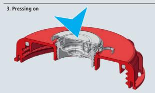
Light pressure on the positioned seal cap makes the locking ring snap into place behind the latching hooks.
